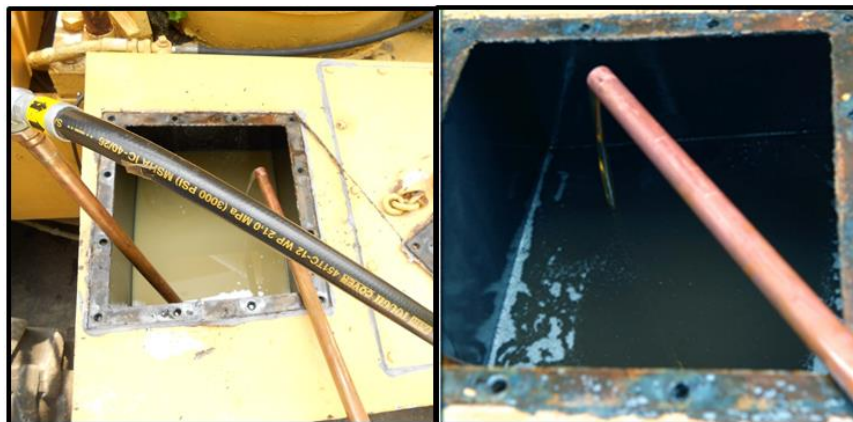
Hydraulic oil before and after dehydration
